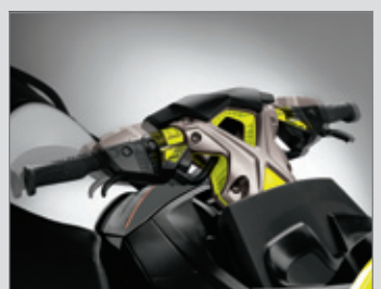
Tilt, racing handlebars with A.E.S. ™
